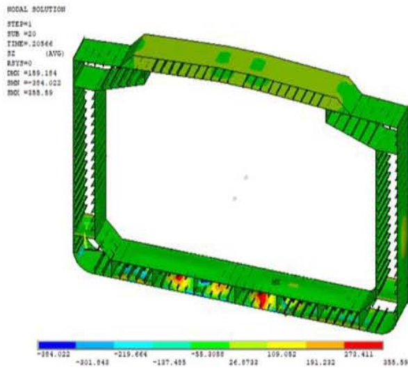
Figure 6. Deformation of FSO at ultimate strength
