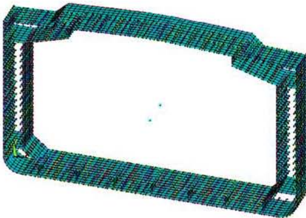
Figure 1. Finite element model of cross section
